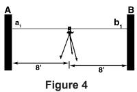
Move the instrument straight towards wall A to a point 2 ft. away and repeat step 2, marking the intersections as a<sub>2</sub> and b<sub>2</sub>, see Figure 5.
